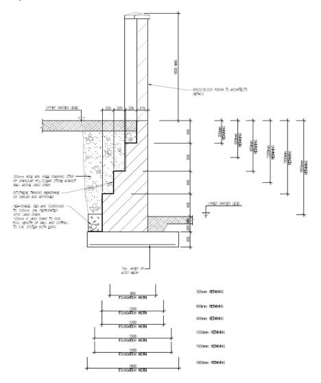
Typical Blockwork Retaining Wall
