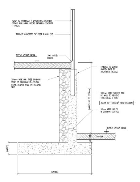
Typical RC Retaining Wall (Up to 3.5m Retaining)
