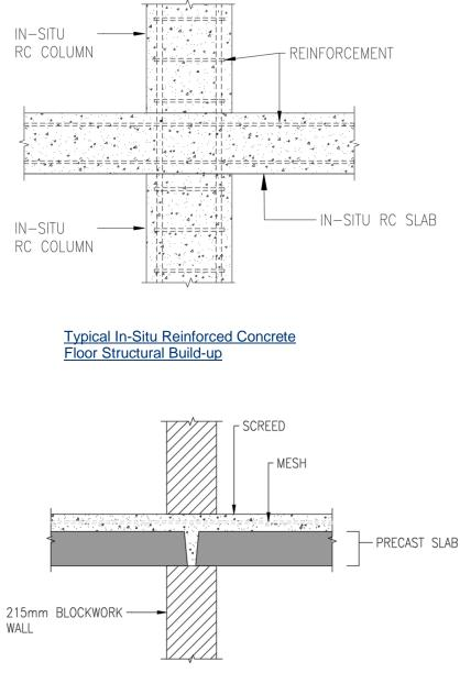
Typical Masonry Walls & Precast Concrete Floor Structural Build-up
